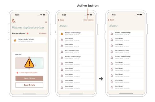
After viewing an alarm, click on "<u>Delete alarms</u>". The cover will not restart until these alarms have been removed.
